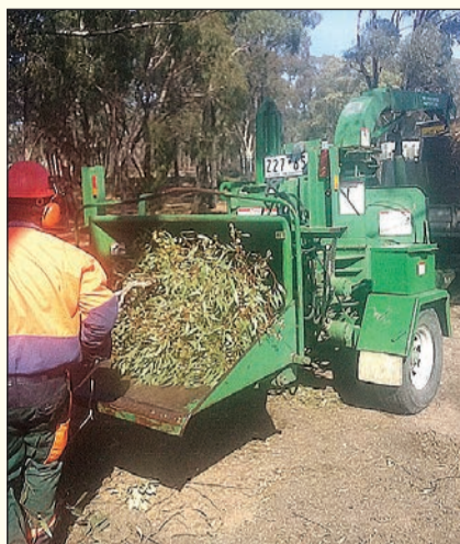
Mulching up to 12' diameter logs on-site
